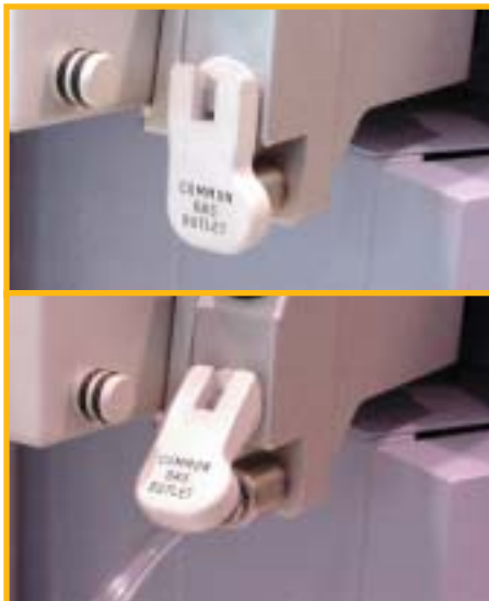
Top: Closed flip-up lid/valve without interlock. Bottom: Open flip-up lid/valve without interlock.
