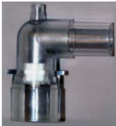
Side view of the Luer adaptor wedged into the elbow of the anesthesia circuit.
