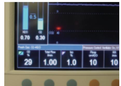
Photograph showing electronic selection of the second gas (e.g., nitrous oxide or air), electronic metering of fresh gas flow (0.7 and 0.3 l/min, respectively), electronic selection of desired oxygen concentration (29%), and the electronic selection of volatile agent (Iso) and desired percent (1.0). Corresponding buttons are depressed, and selections are made with the com wheel (not shown). (This is a photograph of the GE Healthcare, Inc. Aisys anesthesia workstation control panel.)
