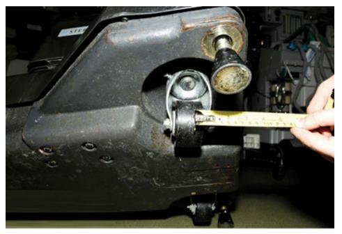
Figure 2: Note that when the OR table's floor locks are released, the fulcrum of the table shifts approximately 3 inches towards the patient's feet. While this is a small shift, it markedly changes the OR table's weight capacity and makes the table prone to tipping.
