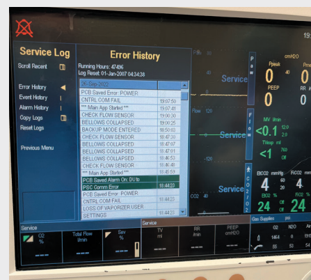
Figure 3: Error log showing "DU to PSC Comm Error" and "POWER CNTRL COM FAIL"
